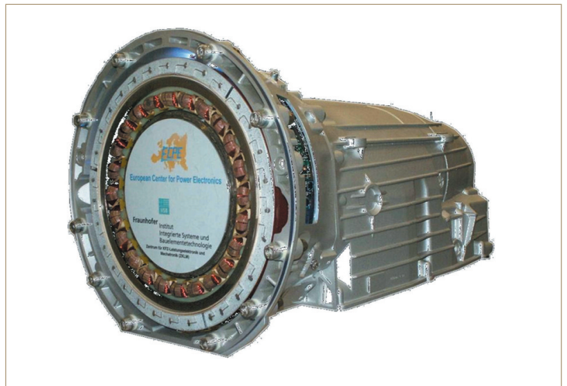
Figure 1: Electric drive with the power electronics, both integrated into the clutch-box screwed at the gear-box
