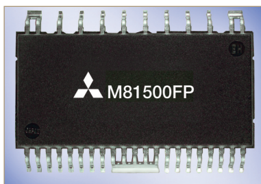
Figure 1: 33pin package of the new SOI single-chip inverter
