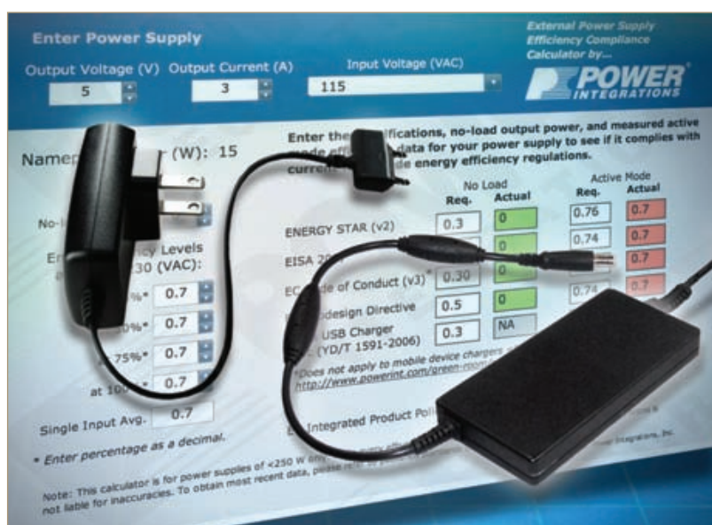
Figure 1: Online tool for calculating power supply conformance to efficiency standards
