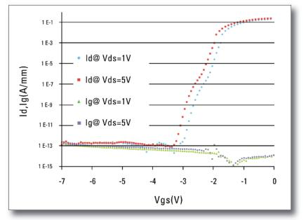
Figure 1: Measured Ia normalised to gate width (850mm) as a function of  $V_{F}$  for  $V_4 = 1V$  and 5V,  $L_4 = 0.3 \mu m$  for LV GaNpowIR device
