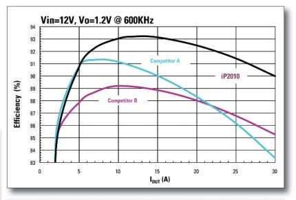
Figure 6: Measured power conversion efficiency for initial GaNpowIR product (iP2010), a  $12V_{\rm m}$  to  $1.2V_{\rm out}$  POL converter power stage operating at 600kHz compared to two Silicon based alternatives
