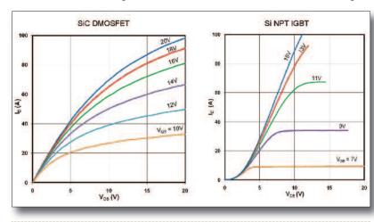
Figure 1: Output characteristics comparison (T<sub>1</sub> = 150°C)
