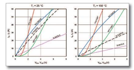
Figure 2: Forward conduction characteristics comparison (Vos = 20V, Voe = 15V)
