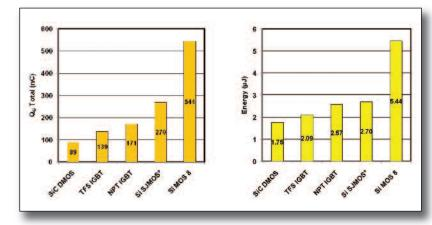
Figure 4: Gate charge and energy comparison
