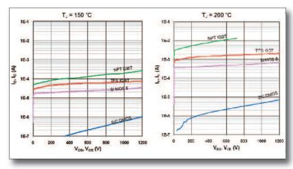
Figure 3: High temperature leakage current comparison
