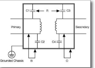
Figure 1: Typical power supply insulation (R location of typical reinforced insulation; B - location of typical basic insulation; O location of typical operational insulation)
