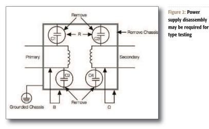
To properly test reinforced insulation the power supply needs to be removed from the chassis. In addition, all paths to chassis ground, as far as practical, need to be removed so as not to over-stress basic and operational insulation during the test.
