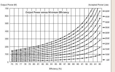
Figure 1: Minimum efficiency required for a given power supply output to ensure compliance with safety standards
