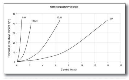
Figure 2: Current vs temperature graph for an example inductor
