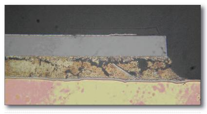
Figure 3: Delamination of solder layer
