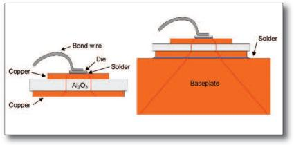
Figure 4: Thermal spreading of DBC (left) and baseplate module
