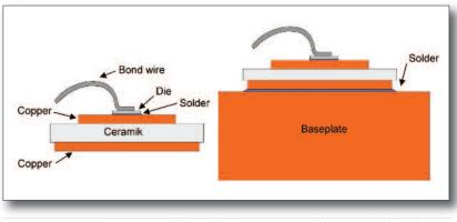
Figure 2: Cross section of DBC and baseplate module
