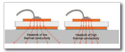
Figure 6: Thermal spreading with low (left) and high conductivity heatsink (water cooled)
