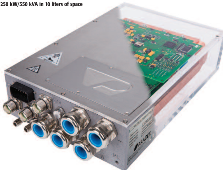
Figure 1: VECTOPOWER featuring peak power of 250 kW/350 kVA in 10 liters of space
