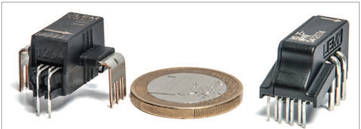
Figure 6: Examples of two different current transducers using the described ASIC
