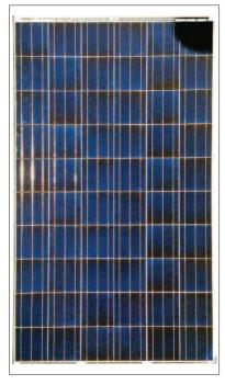
Figure 3: Solar panel shaded in top right corner
