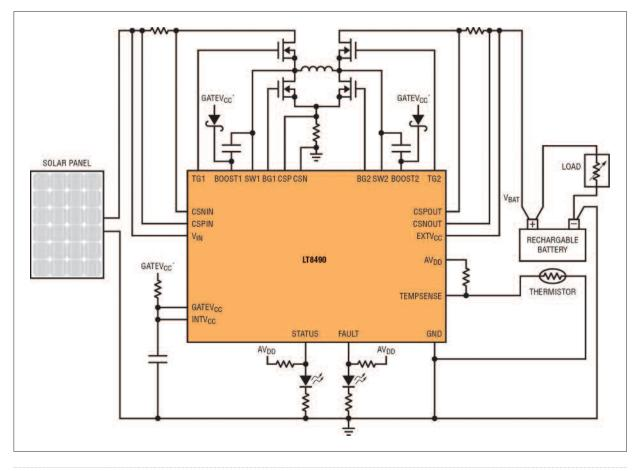
Figure 1: Simplified solar powered battery charger schematic
