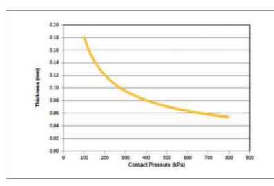
Figure 3: Thickness vs. pressure of TIM HT-C3200
