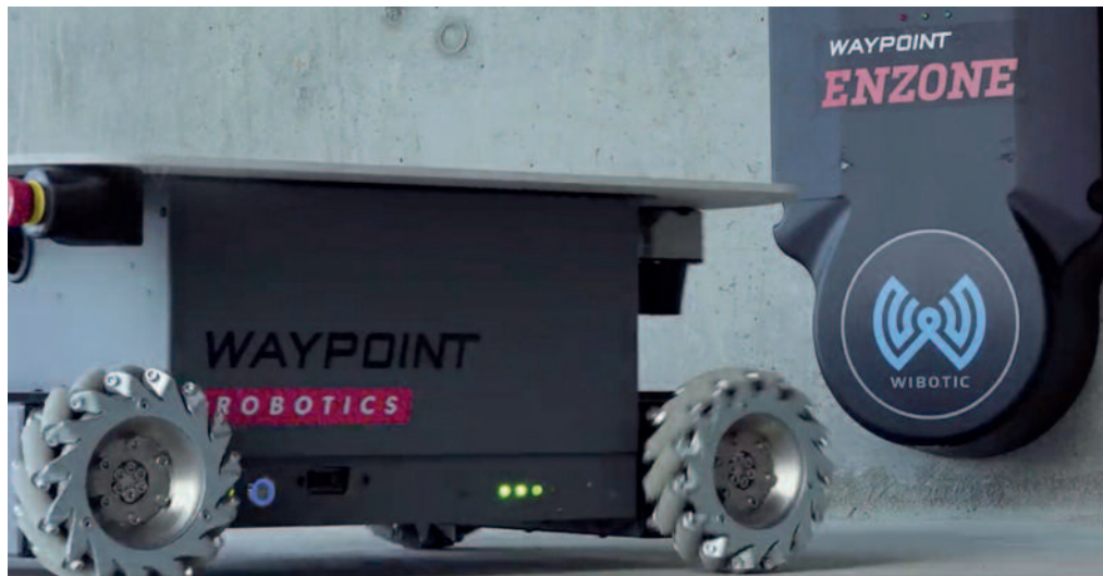
Figure 4: Wireless power transfer in robotics enables high autonomy
