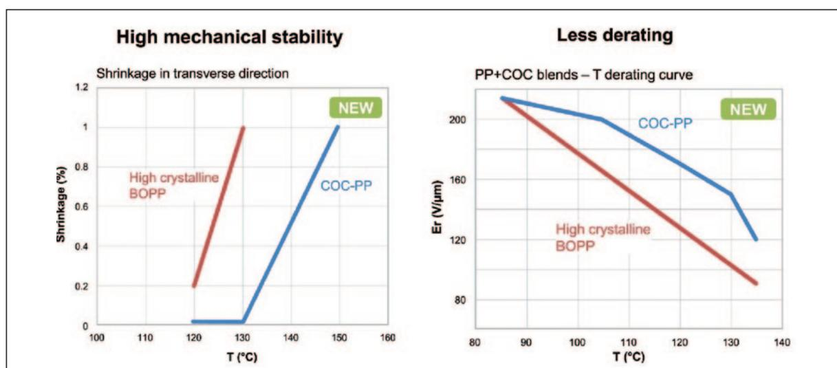
Figure 1: At temperatures of up to 130°C the new COC-PP material exhibits no shrinkage in a transverse direction (left), voltage derating of the new material is also significantly better (right)
