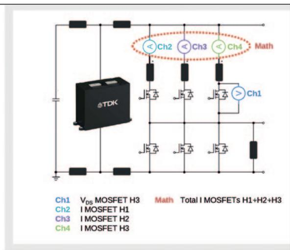
Figure 5: The new HF film capacitor series features extremely low voltage overshoot and ringing
