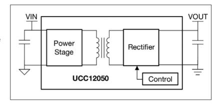
Figure 6: UCC12050 isolated DC/DC bias power supply
