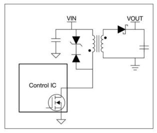
Figure 2: Simplified schematic of the flyback converter
