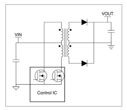
Figure 4: A push-pull transformer driver
