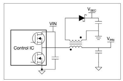
Figure 3. A Fly-Buck™ converter
