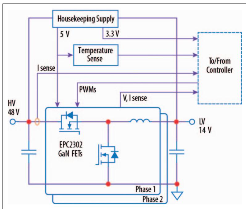
**Figure 1: Simplified schematic diagram of the multi-phase bi-directional converter**
