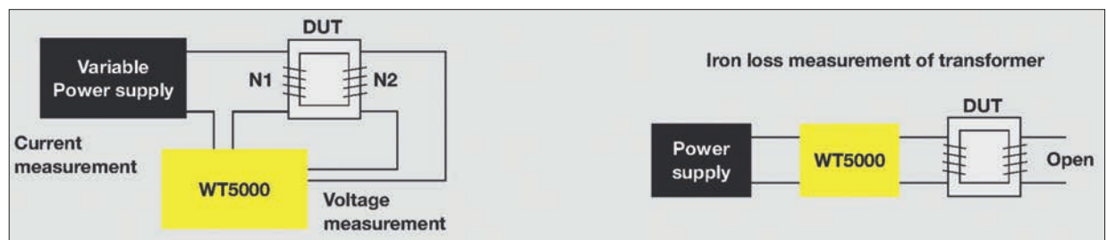
BELOW Figure 7: In transformer or reactor development, the WT5000 can be used to evaluate magnetic material characteristics using Epstein frame system
