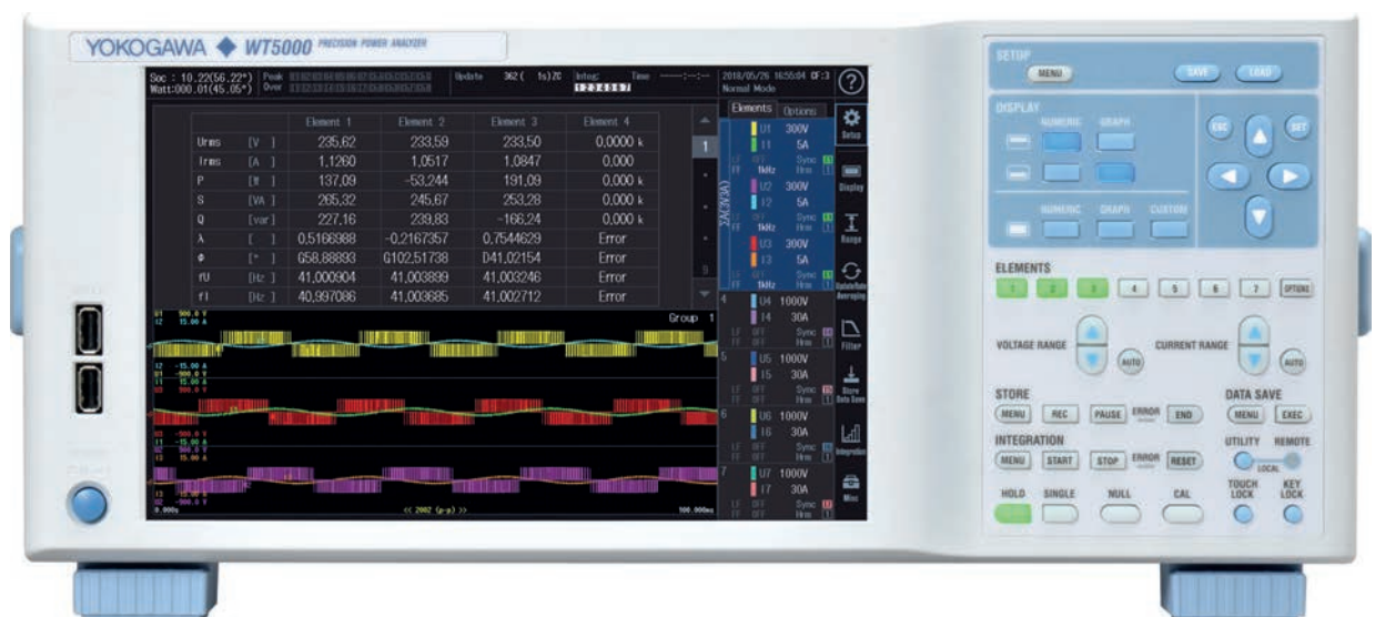
Figure 1: Operable by touch and/or hardware hot-keys independently, up to 7 different power phases at 10 MS/s (18 bit) can be measured on the 10.1 inch screen
