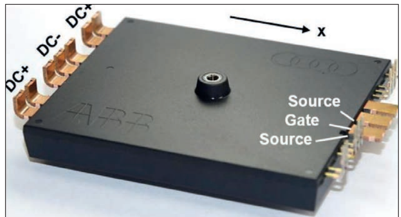
Figure 2: 1200 V SiC and Si mold module, Gen 2 design
