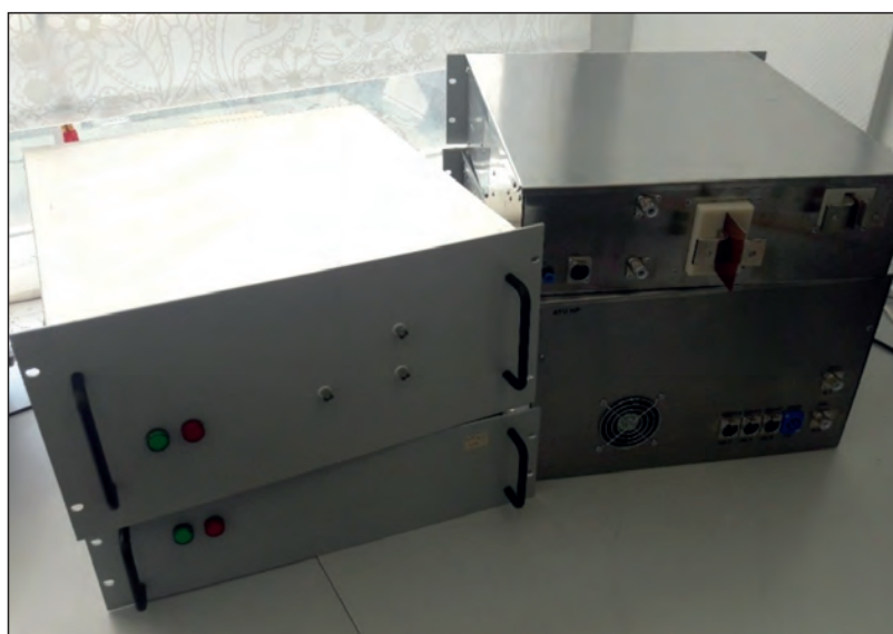
Figure 2: Measuring and auxiliary units are designed for a standard 19" rack
