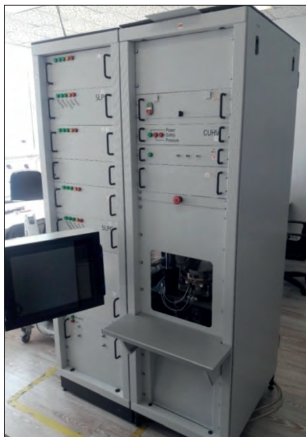
Figure 1: Newly test system for comprehensive measurements on bipolar power devices
