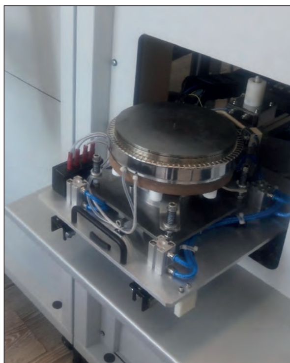
Figure 3: Draw-out loading system allowing to easily install a large-diameter device or a device in hot state
