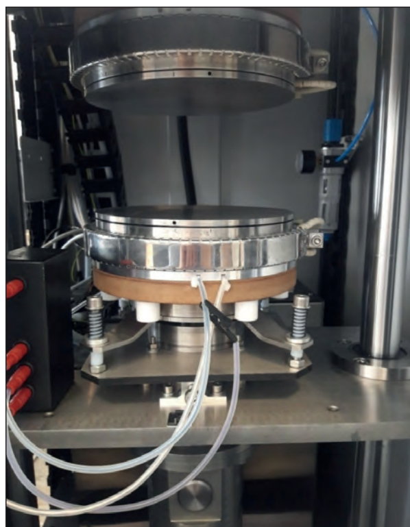
Figure 4: The clamping system feature replaceable upper and lower contact surfaces
