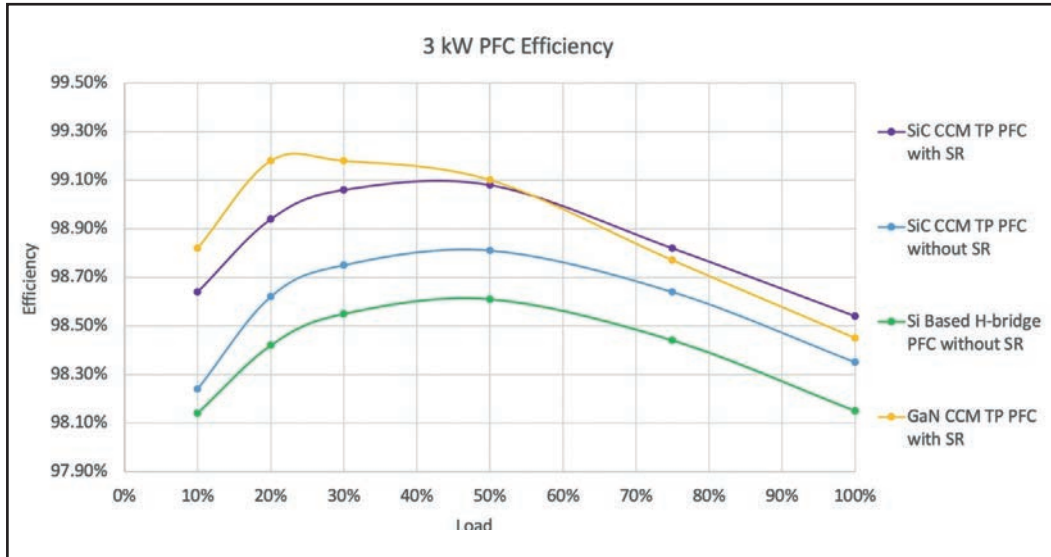
Figure 6: Silicon Carbide is the best choice in a totem pole PFC, especially for high reliability applications
