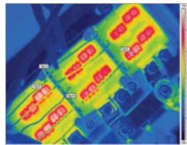
Figure 9: Infrared measurement of power module while operating all IGBTs
