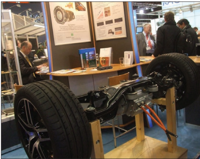
New highly integrated electrical drive for (hybrid) electric vehicles driving directly front wheels
