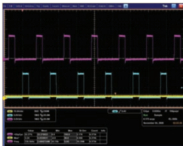
Figure 6: Switch nodes signal (Channel 2 and Channel 3) and current (Channel 1) at the end of the charging cycle
