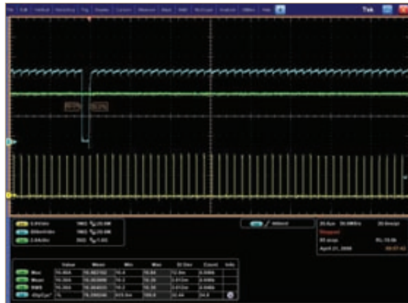
Figure 3: Constant short circuit at 10A. CHANNEL 2 (blue) shows the UVLO pin that is pulled down after 256 cycles; CHANNEL 4 (green) shows the output current equal to the current limit 10A; CHANNEL 1 (yellow) shows the drain voltage
