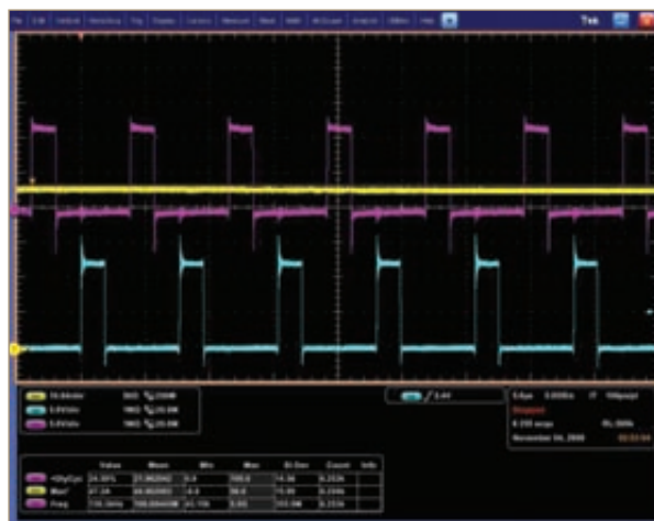
Figure 5: Switch nodes signal (Channel 2 and Channel 3) and current (Channel 1) when the voltage across the Boostcap is 2.5V
