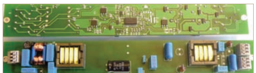
Figure 6: Bottom and top side of fully featured demo board for ICB2FL01G lamp ballast controller
