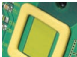
Gap Filler I500 has natural tack and cleanly flows into position for final assembly without leaving thermal material behind.
