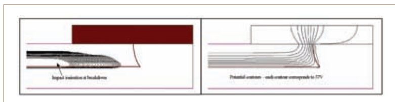
Figure 4: Forward diode impact ionisation (left) and reverse diode potential contour at a breakdown voltage of 375V
