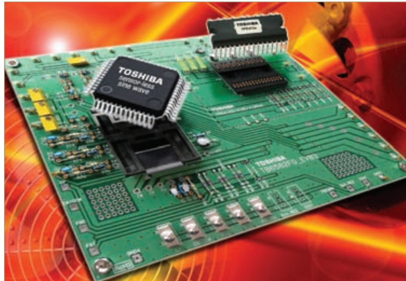
Figure 4: Evaluation platform featuring single-chip inverter and controller that will simplify and speed the development of BLDC motor drives
