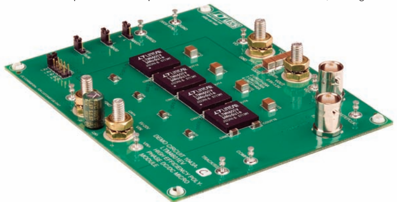
Figure 1: Four DC/DC μModule regulator systems current share to regulate 1.5V at 48A with only 2.8mm profile and 15mm x 15mm of board area
