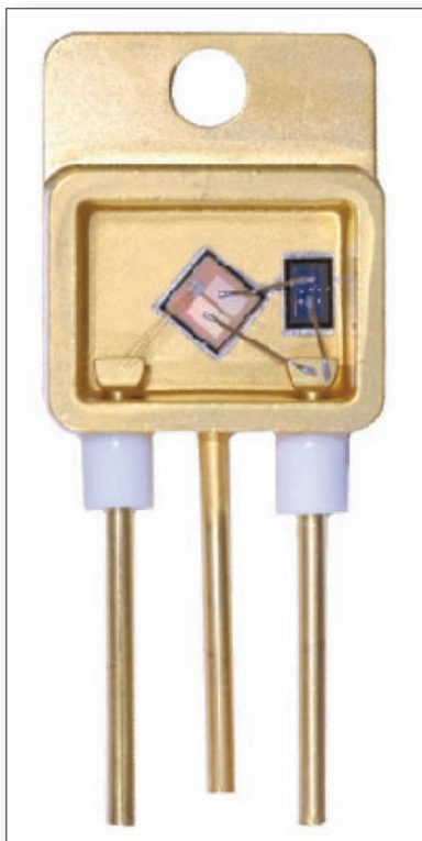
Figure 1: 1.7kV SiC MOSFET with 1.7kV, 10A JBS diode in TO-258 package co-pack
