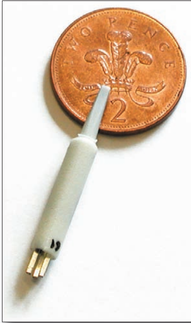
Figure 2: Miniature fluxgate magnetometer for the I-prober 520
