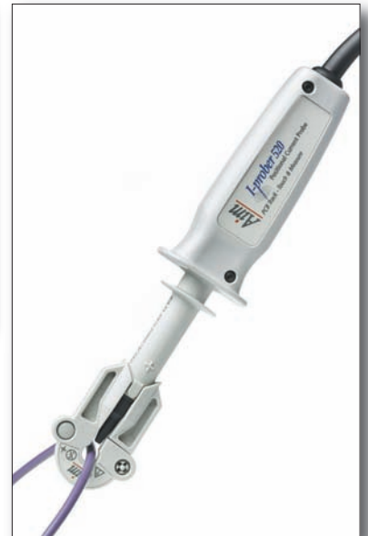
Figure 5: Measuring wire current
