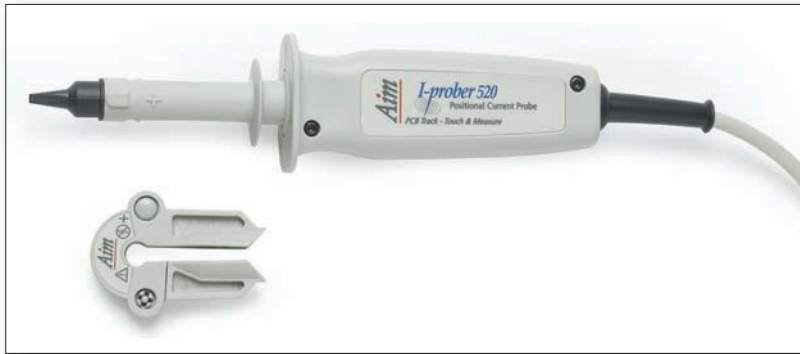
Figure 4: Clip-on toroid assembly for measuring current in a wire
