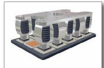
Figure 4: Press-pins contact the emitter side of the IGBT chip
