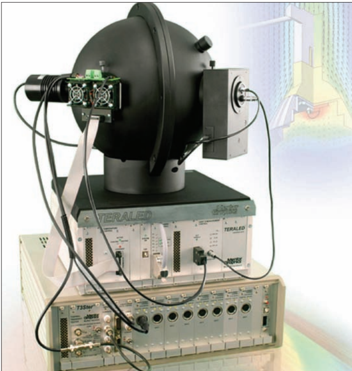
T3Ster and TERALED together provide a comprehensive solution for LED testing
