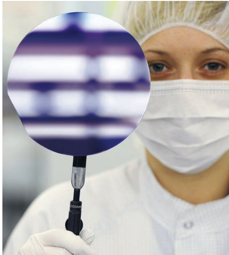
First gallium-nitride LED chips on 6" silicon wafers in pilot stage at Osram Semiconductors
