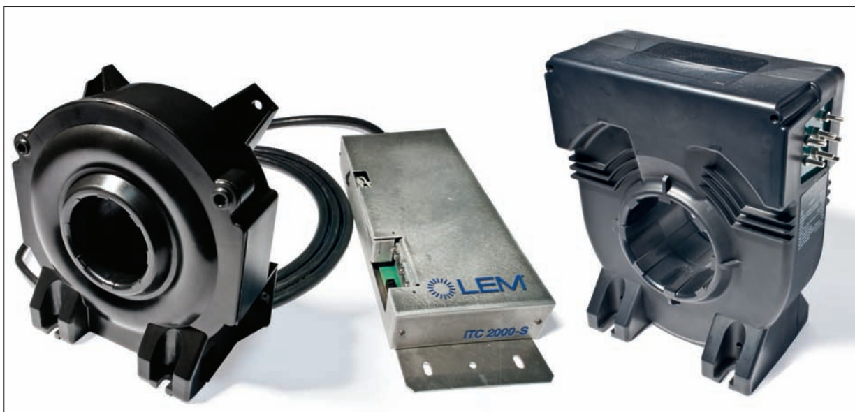
Figure 1: The ITC current transducer series; the variant with remote signal processing module (left) facilitates mounting in traction-unit roof voids
