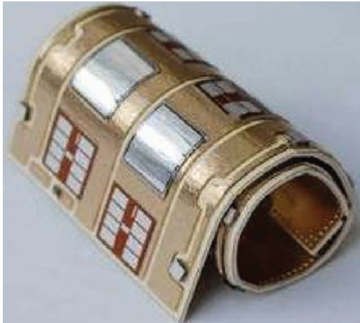
Figure 3: DBC substrate after mechanical stress test
