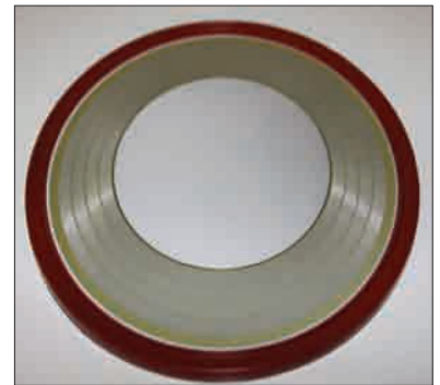
Figure 9: Prototype of 150mm 4.5 kV RC-IGCT
