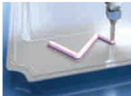
Gap Filler I000SR dispenses into position without slumping. With minimal pressure, flows in place with little to no stress on components.
