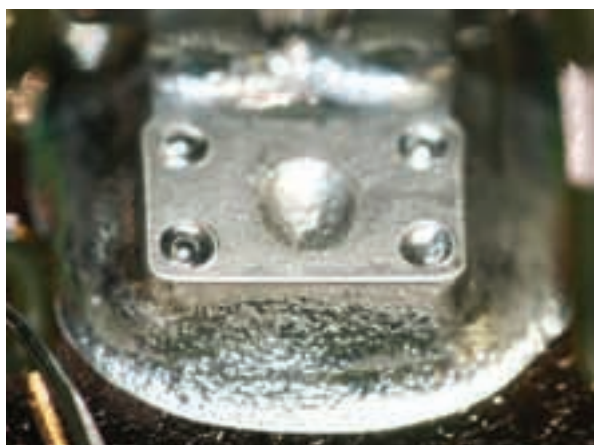
Figure 4: Improved main terminal foot
