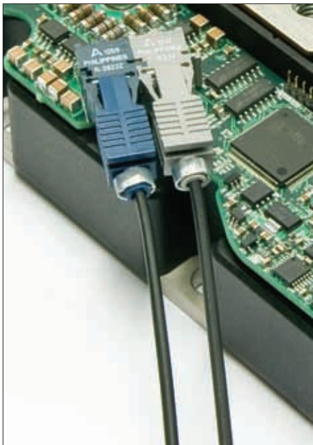
Amantys' IGBT driver Power Insight™ protocol runs over Avago's 50 MBd Versatile Link™ transmitters and receivers
