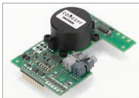
CT Concept's driver core for IGBT modules with blocking voltages of 4.5 kV and 6.5 kV
