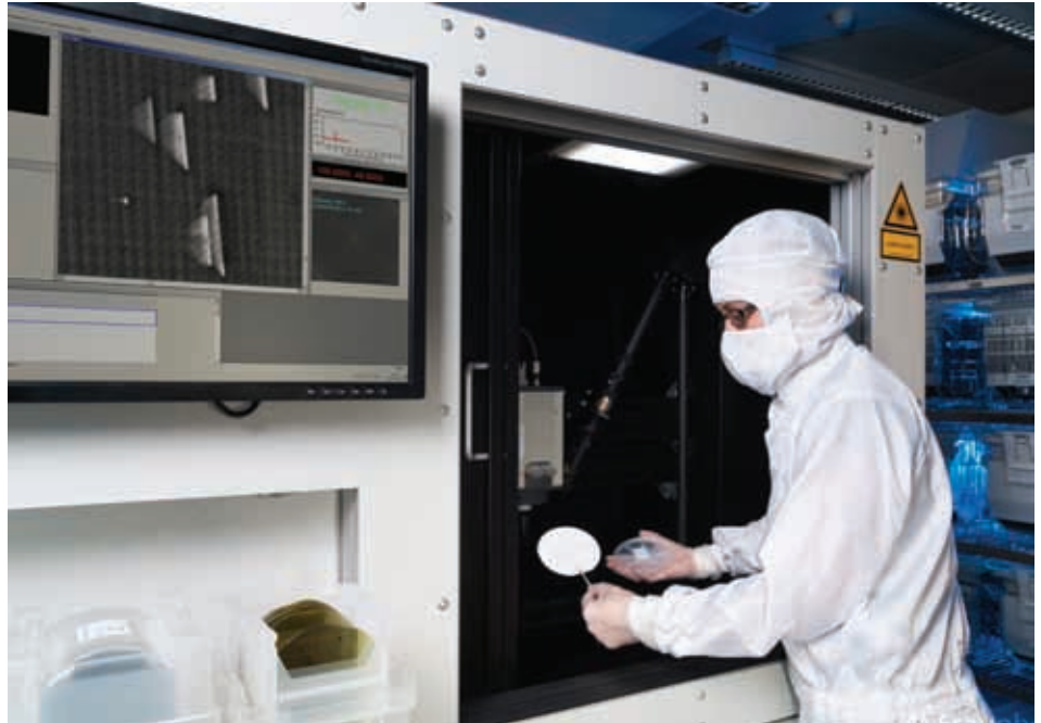
Operator loading a 100 mm SiC epiwafer in the defect luminescence scanner at Fraunhofer IISB
