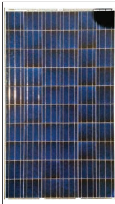
Figure 3: Solar panel shaded in top right corner
