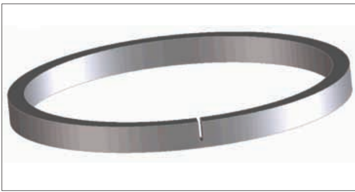
Partial air gap on magnetic core
