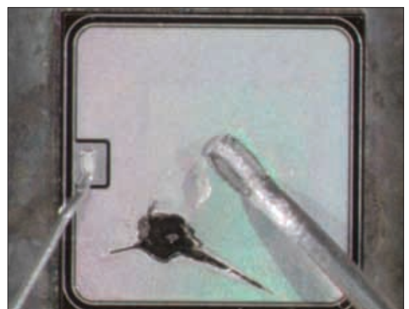
RIGHT Figure 6: SiC MOSFET destroyed by cosmic ray failure Source: ST Microelectronics
