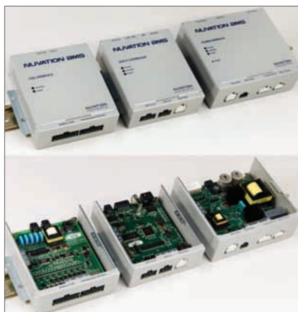
Figure 2: The three major subsystems of the Nuvation BMS - cell interface, stack controller, power interface - comprise a modular, hierarchical design which results in scalability, robustness, and reliability across a wide range of power levels as shown in the block diagram (above) and physical realization (right)
