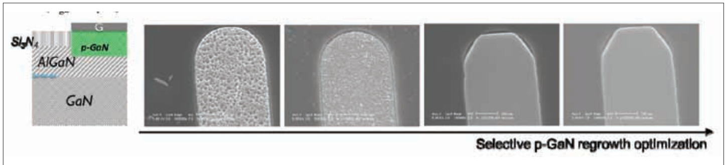
Schematic cross-section (left) and first optimization tests of selective p-GaN re-growth
