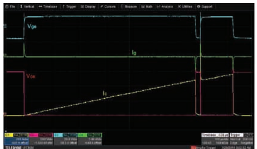
Figure 5: 1500 V/600 A double pulse waveform on a FZ1200R33KF2 IGBT module
