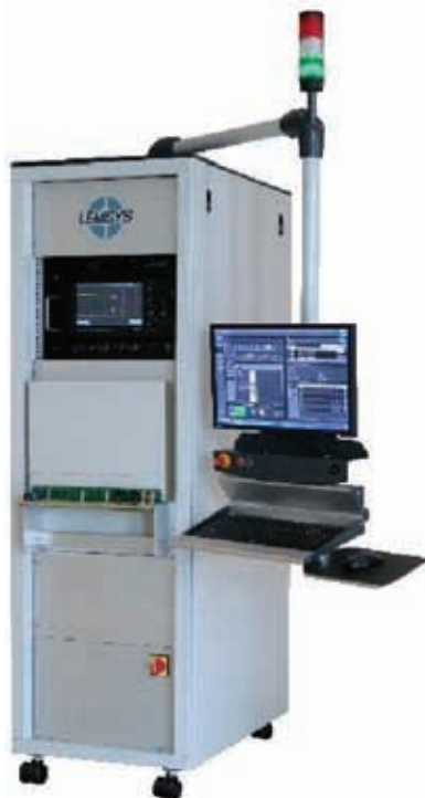
Figure 1: Lemsys new Pro-AC power semiconductor test equipment
