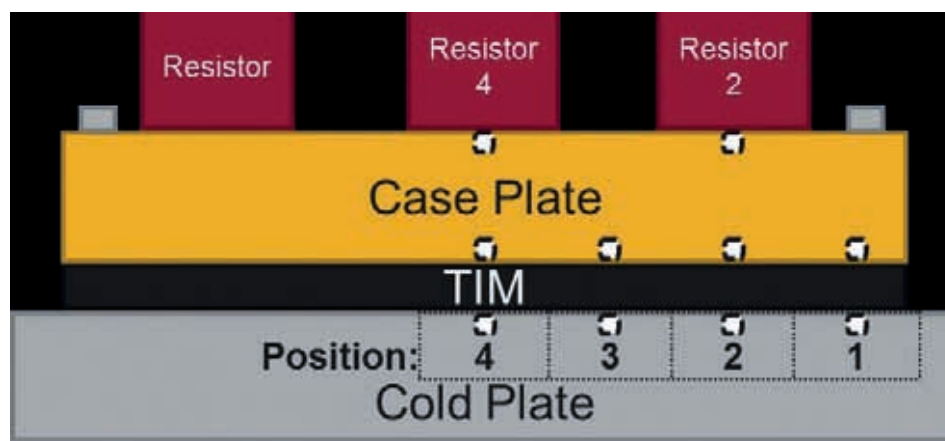
Figure 1: Schematic and temperature measurement locations in the assembly
