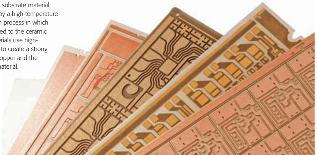
Figure 1: The four curamik ceramic circuit materials provide different levels of thermal dissipation
