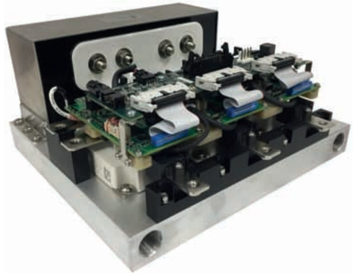
Mersen's SiC reference design is built around a 3-phase, 700 VDC / 200 A water-cooled converter
