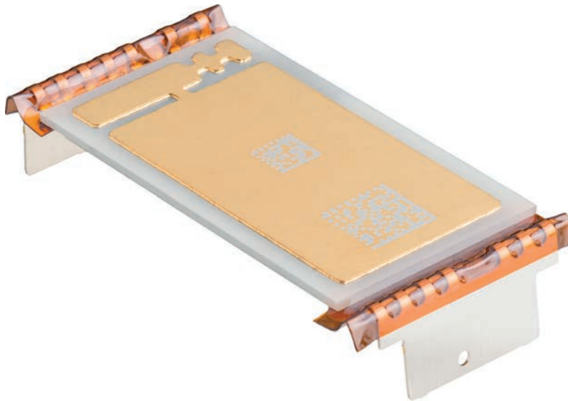
Figure 4: The 650 V, 1.7 m \Omega , 750 A Delphi SiC module contains five 650 V, dual-side sintered, 7 m \Omega SiC MOSFETs in a single switch configuration
