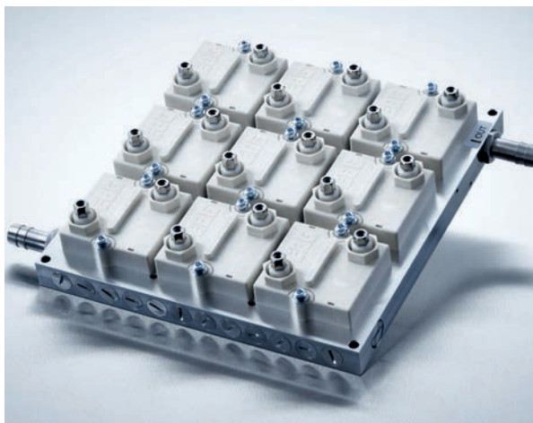
Figure 2: Resistor heat-sink unit for industrial filter application (left), and resistor with preapplied PCM (phase change material)
