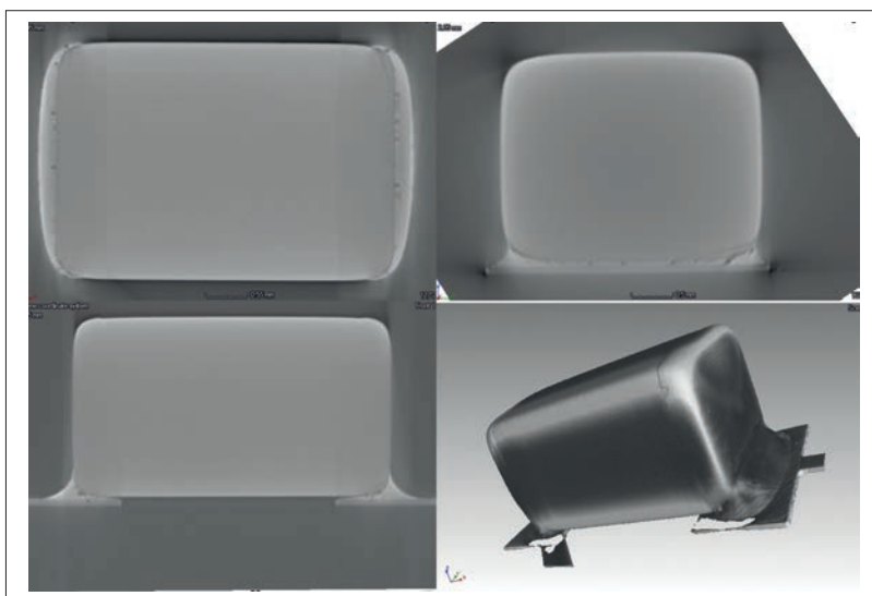
Figure 10: Non-destructive virtual 3D slicing images and 3D reconstruction of the cracked MLCC from Figures 4 to 6 for even better crack identification
