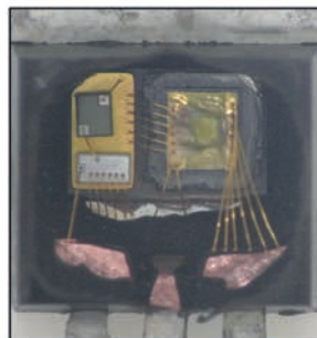
Transphorm Cascode configuration
