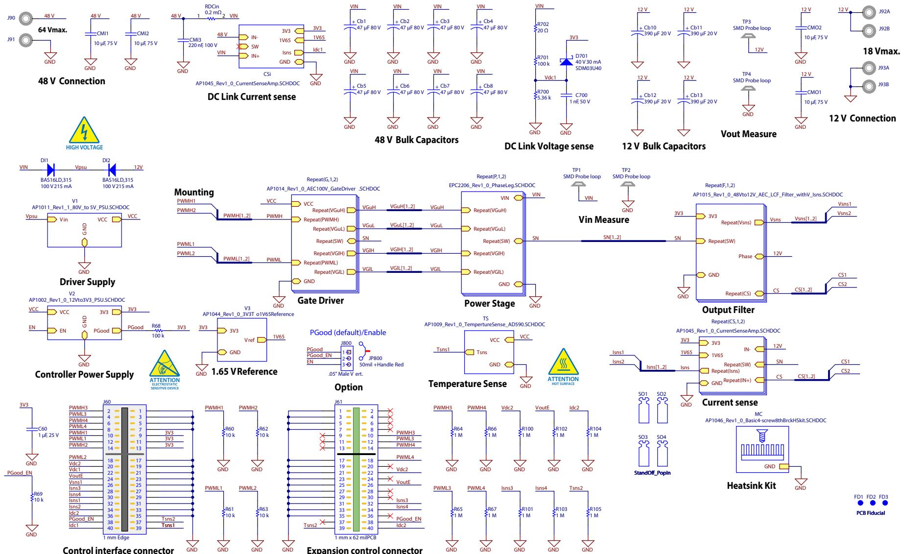
Figure 8: EPC9137 Rev 4.0 main schematic
