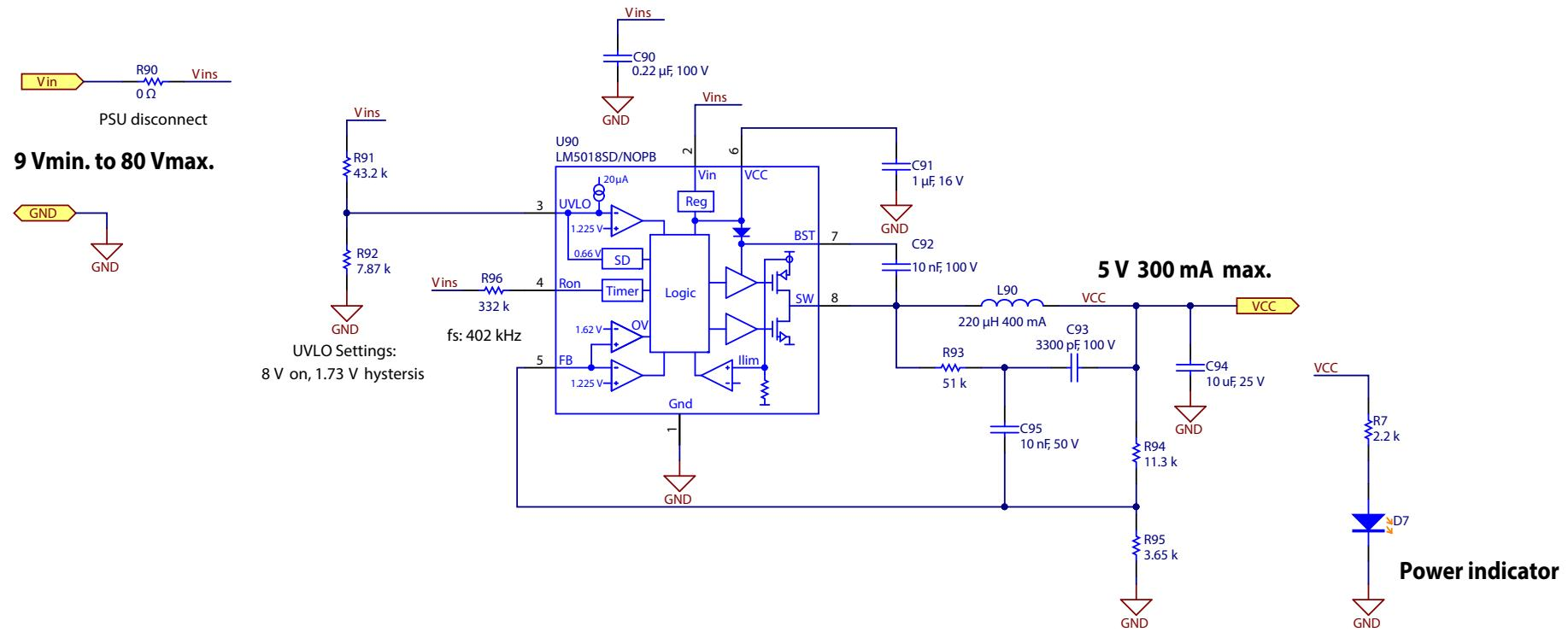
Figure 9: EPC9137 80 V to 5 V housekeeping power supply
