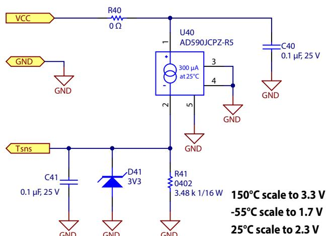
Figure 16: EPC9137 AD590 temperature sense
