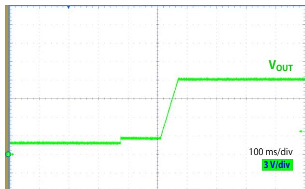
Figure 4. Buck converter output voltage start up response
