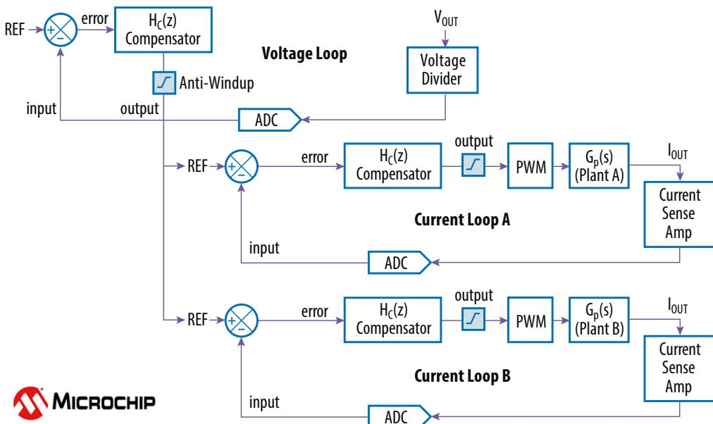
Figure 5. Interleaved buck converter average current mode control
