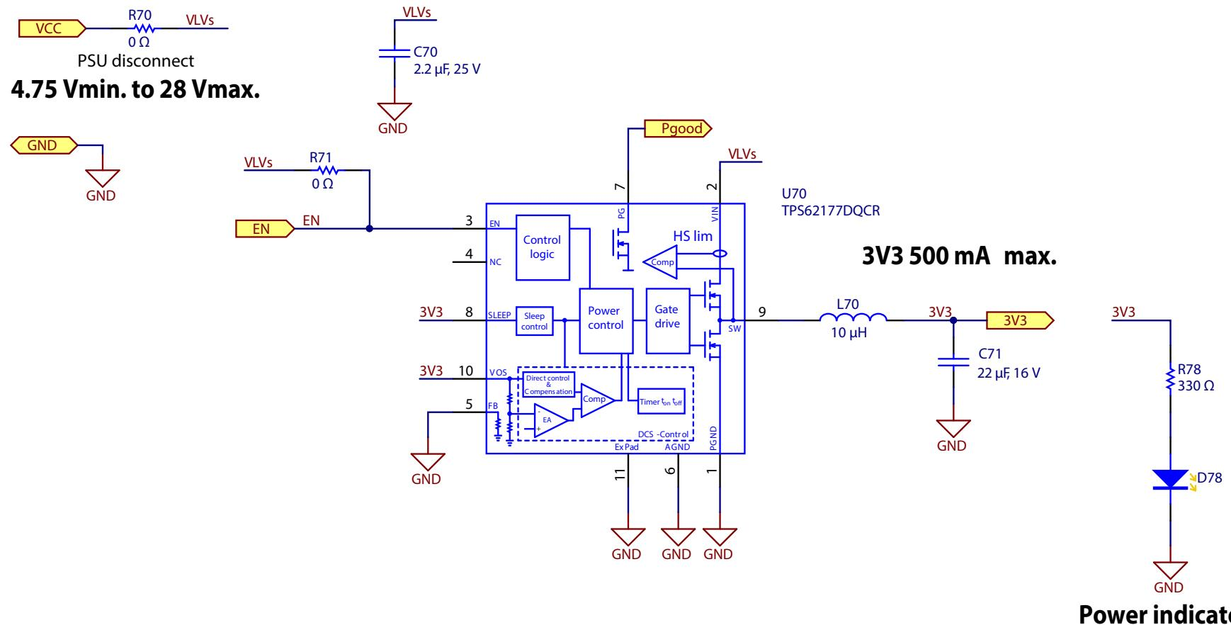
Figure 10: EPC9137 3V3 housekeeping power supply
