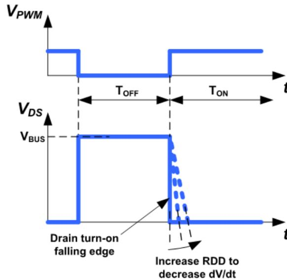
**Fig 12.** Turn-on dV/dt slew rate control simplified timing diagram
