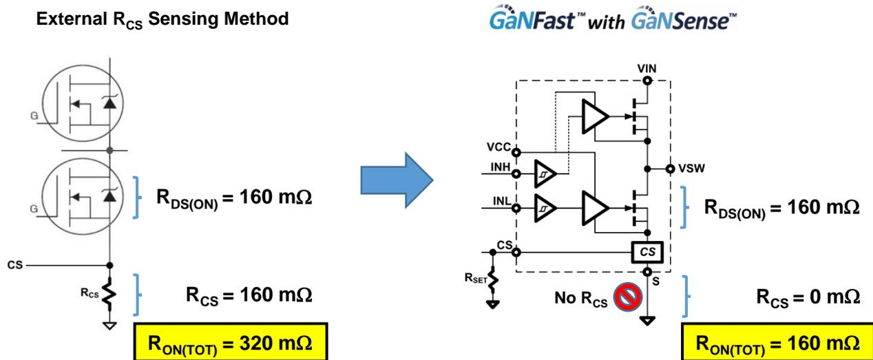
**Fig 8.** External resistor-sensing vs. GaNSense loss-less current sensing
