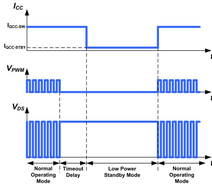
**Fig 14.** Autonomous low-power standby mode timing diagram
