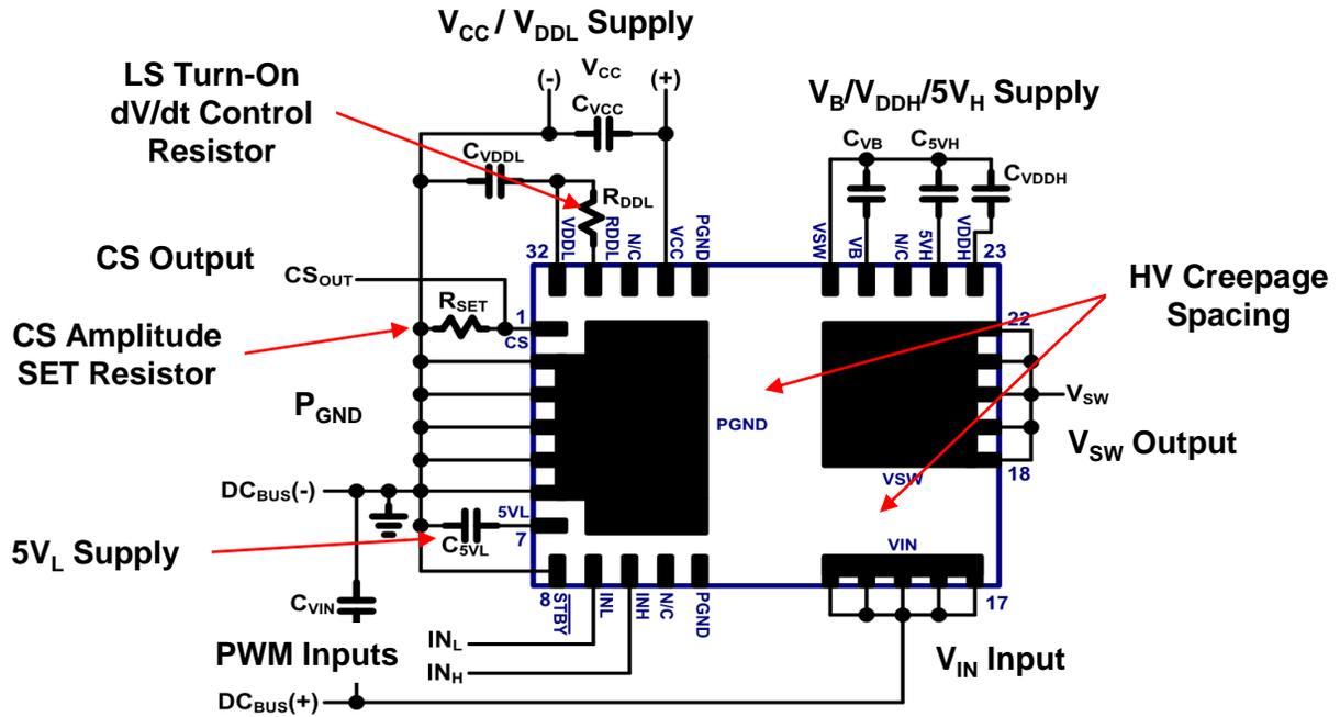
**Fig 3.** IC connection diagram
