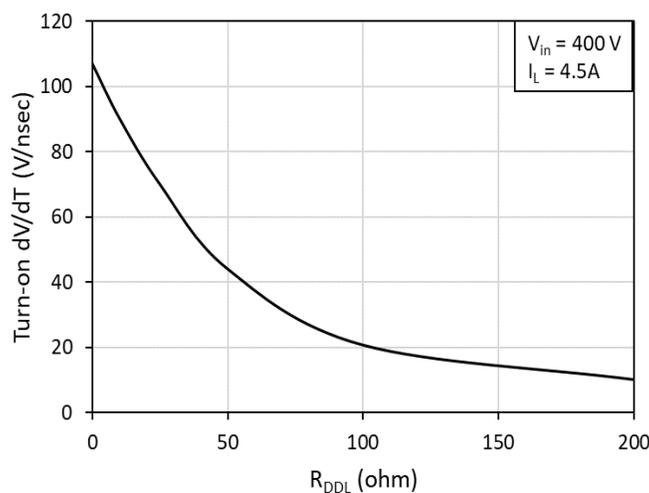
**Fig 13.** Low-side  $V_{DS}$  turn-on slew rate (dV/dt) vs  $R_{DDL}$  curve
