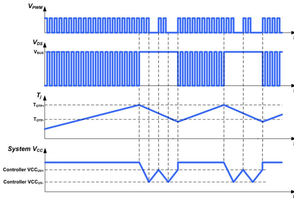
Fig 11. OTP timing diagram
