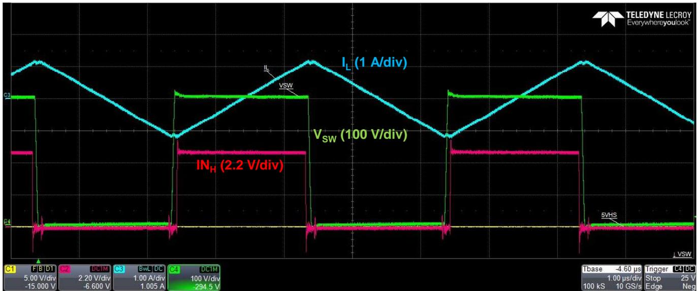
**Fig 5.** GaNFast Half-Bridge IC basic switching waveforms (resonant ZVS mode, duty-cycle = 50%,  $F_{SW} = 250$  kHz)
