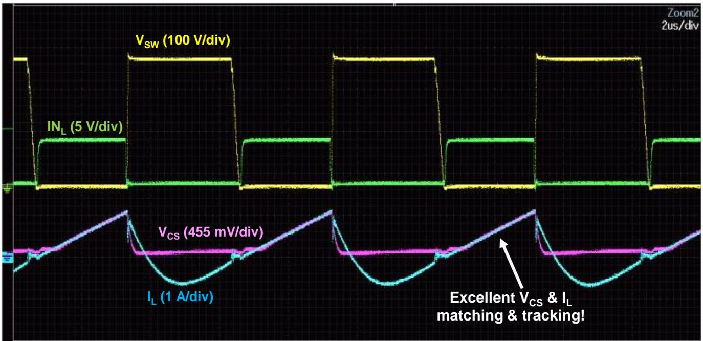
**Fig 9.** Loss-less current-sensing waveforms
