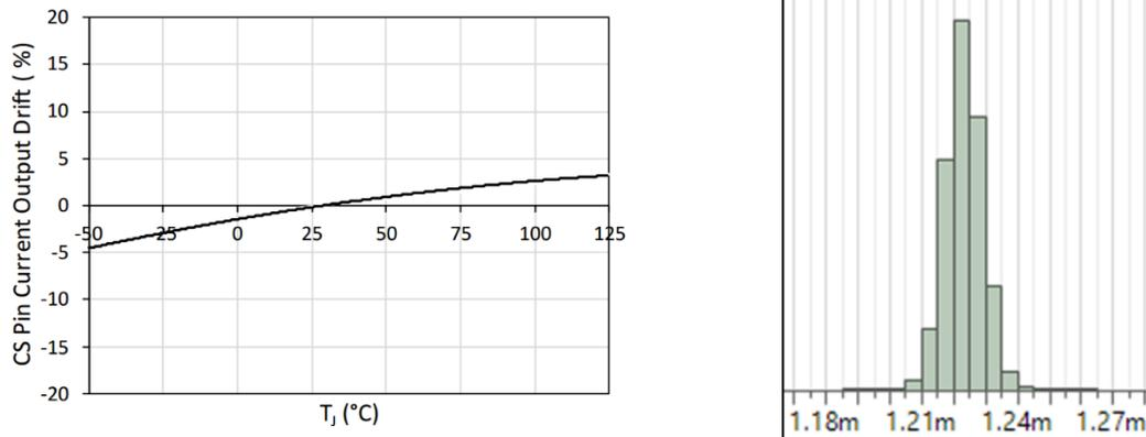
**Fig 7.** CS pin current vs  $T_{CASE}$  and post-trim production data (typical only)
