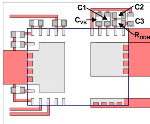
Fig 17. NV6245C and NV6247 dual-PCB footprint layout
