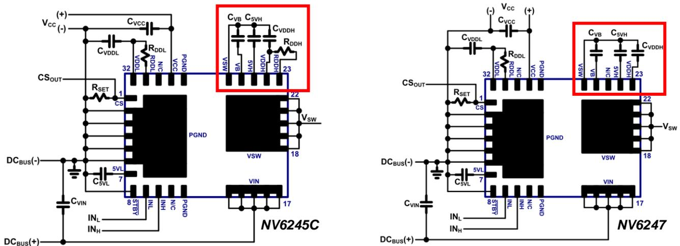
Fig 16. NV6245C and NV6247 IC connection diagrams
