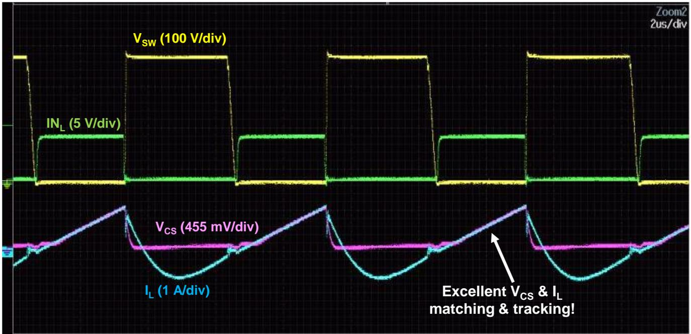
**Fig 9.** Loss-less current-sensing waveforms
