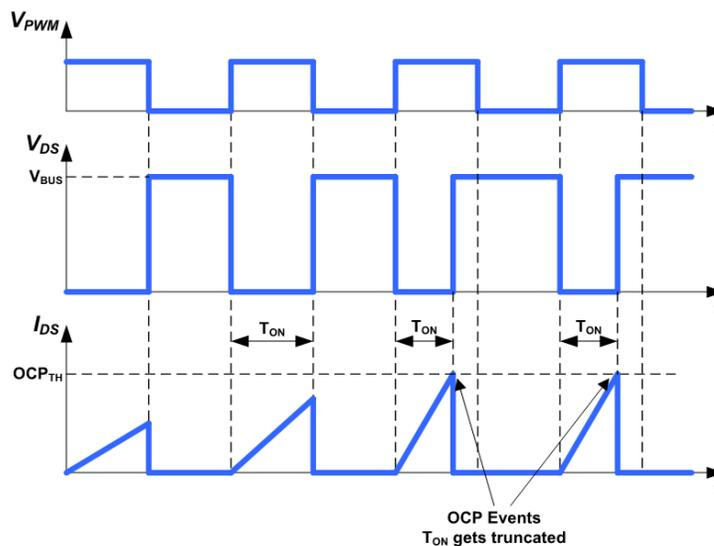
**Fig 10.** OCP timing diagram
