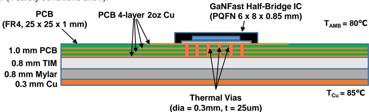
**Fig 20.** Bottom-cooled thermal-model stack-up diagram
