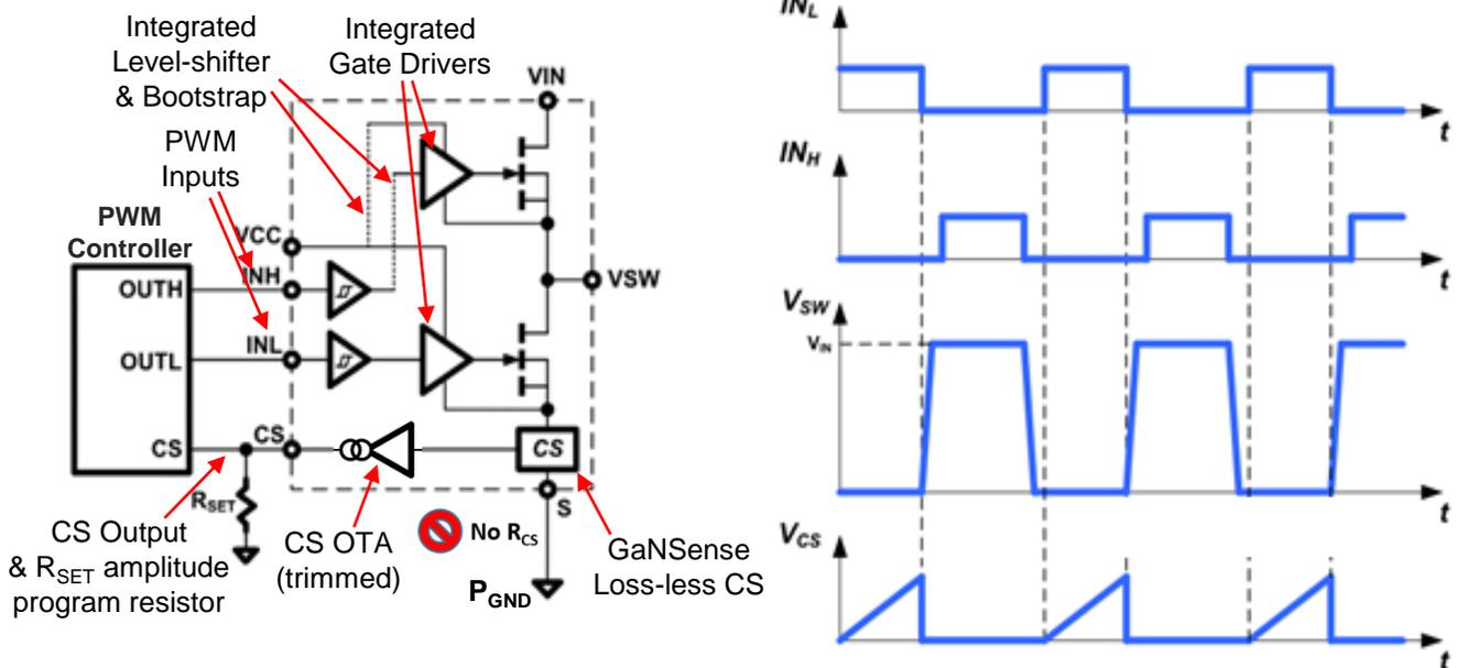
**Fig 6.** IC simplified internal block diagram & timing diagram
