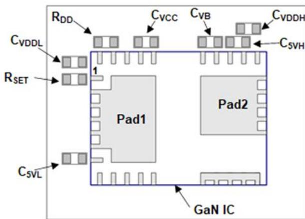
Step 1. Place GaN IC and components on PCB. Place components as close as possible to IC
