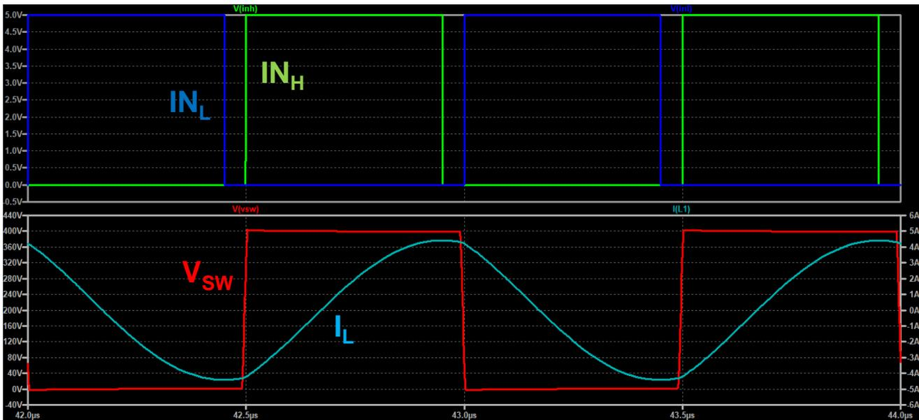
**Fig 18.** Electrical-simulation model & ZVS resonant circuit and simulation waveforms
