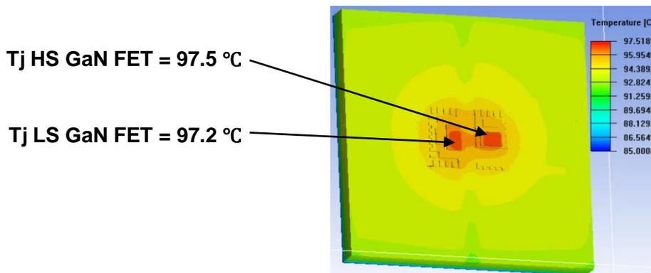
**Fig 21.** 3D thermal simulation results
