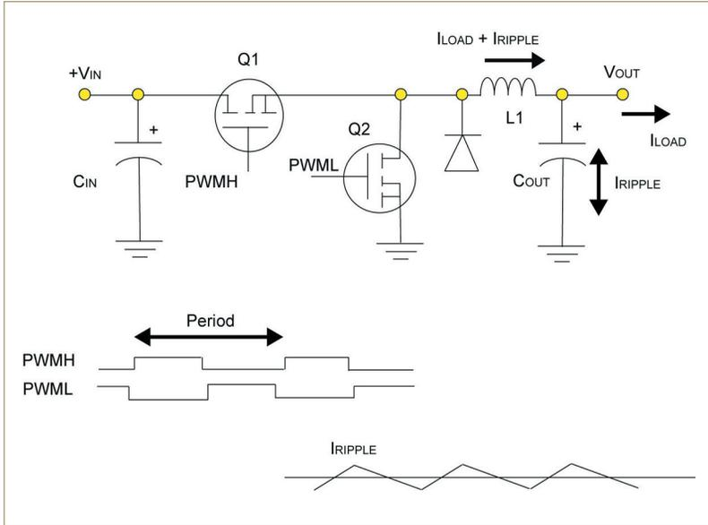
Figure 3: Synchronous buck converter
