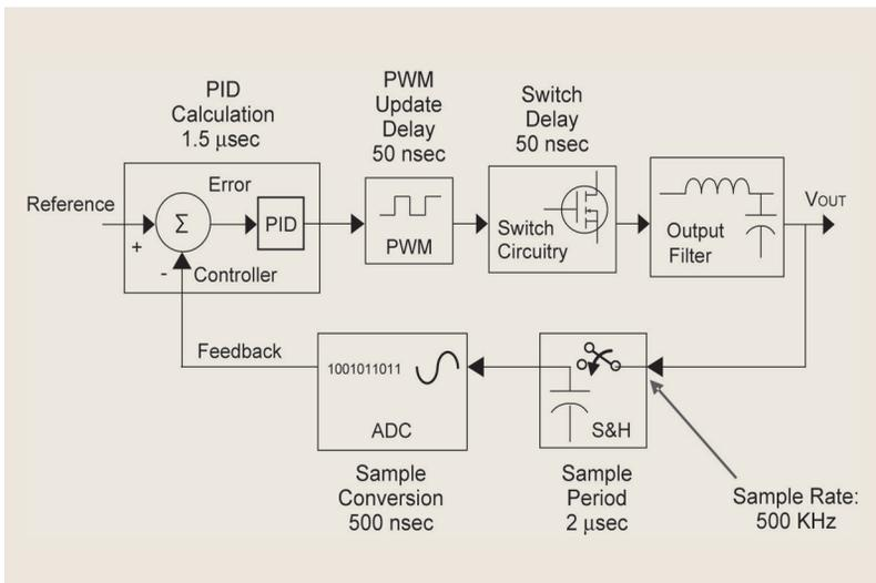
Figure 4: Example SMPS control system
