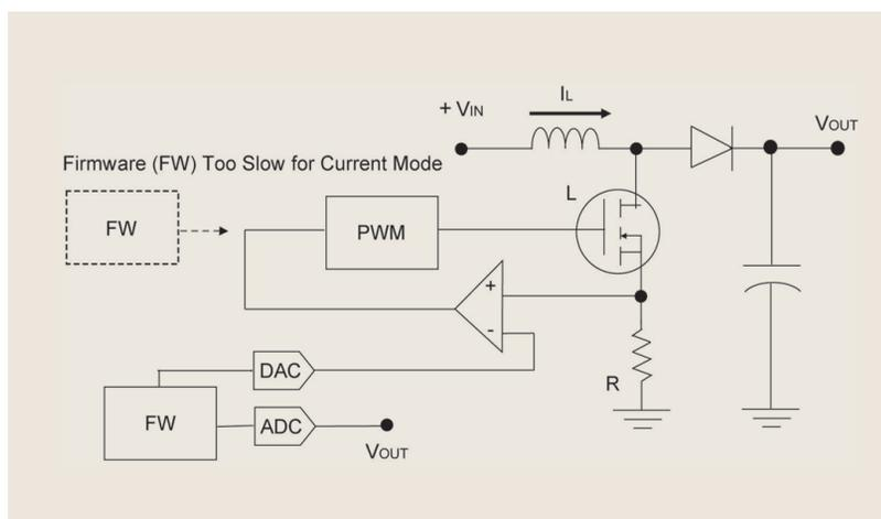
**Figure 6: Current limiting using analogue comparator**
