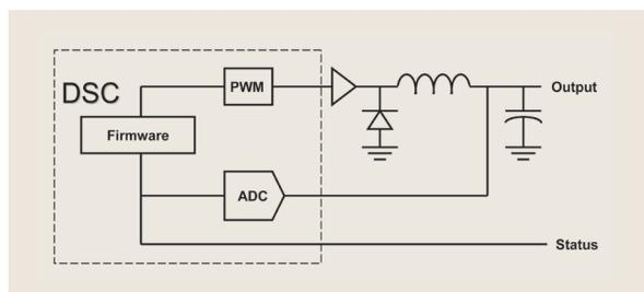
**Figure 1: Example of a digital loop architecture**
