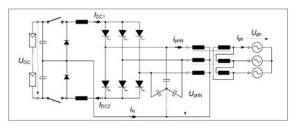
Figure 1: Inverter topology (Minnesota Inverter) with six thyristors and two HF-switches (IGBT or SiC MOSFET)
