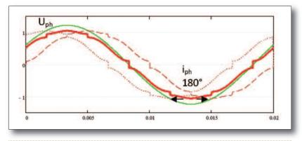
Figure 3: Output voltage and phase shifted output currents of transformer
