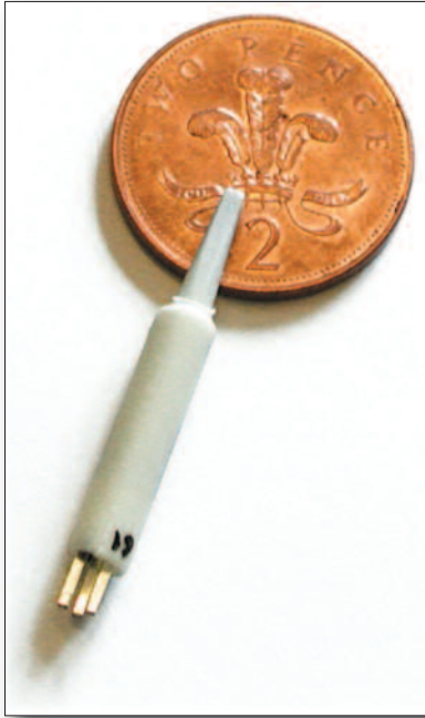
Figure 2: Miniature fluxgate magnetometer for the I-prober 520
