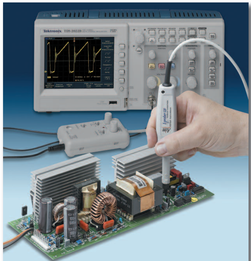
Figure 1: New current probes allow for direct current measurement up to 20 A in PCB tracks of power supplies
