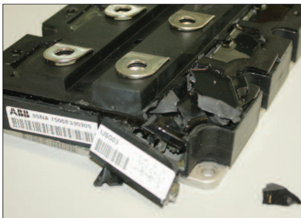
Figure 2: Old HiPak 2 module after destructive short-circuit test (left) and improved HiPak 2 module after same test
