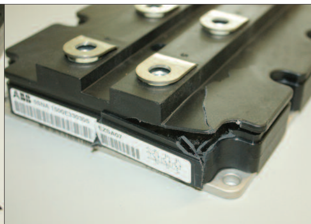
Figure 2: Old HiPak 2 module after destructive short-circuit test (left) and improved HiPak 2 module after same test
